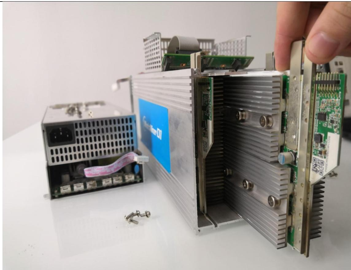
2) After installing the hash board into the chassis, first install the adapter board. The socket of the adapter board and the pin of the hash board must be installed in place to avoid other problems caused by contact problems, as shown:
