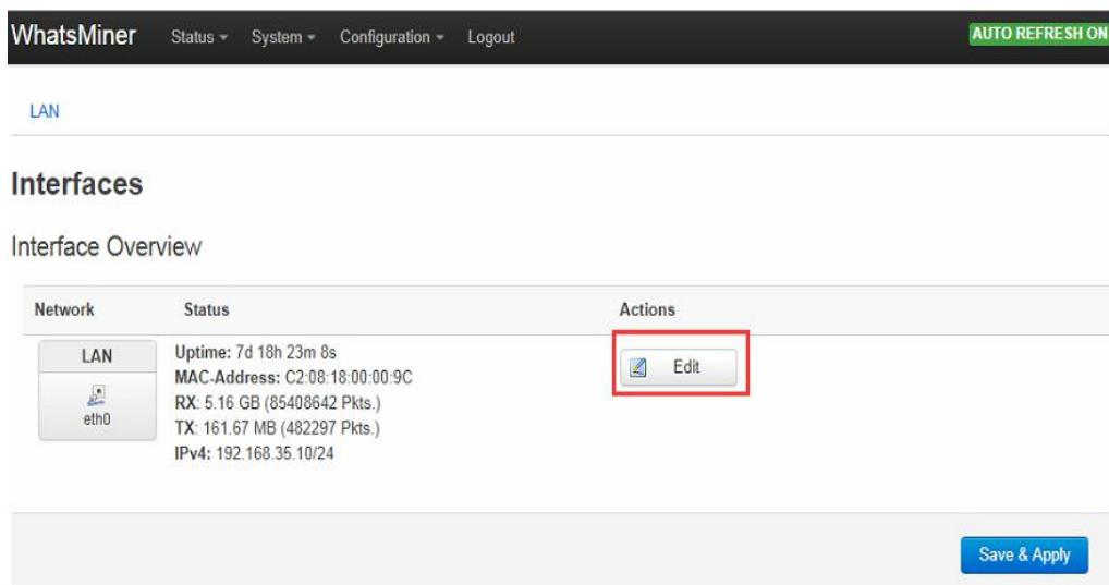
The screenshot shows the 'Edit' interface for the LAN network card. The top navigation bar is identical to the previous screenshot. The main content area is titled 'Interfaces' and contains a 'Interface Overview' table. The 'LAN' (eth0) row is selected and has a red box around its 'Edit' button in the 'Actions' column. The 'Save & Apply' button is visible at the bottom right.
